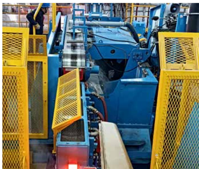
The HAZELETT twin-belt copper bar caster
